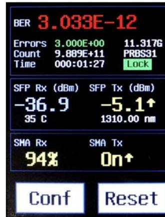
Upon exiting the configuration screen, the Eye-BERT begins monitoring and displaying the bit error rate on the selected interface along with the optical and electrical interface status and measurements.
